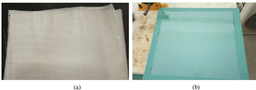
Fig. 1. Manufacturing and Fabrication (a) Unidirectional plain weave (b) Mylar sheet used as mould releasing agent
